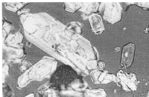
Fig. 1a Slow formation of a new very insoluble crystalline modification during storage of a liquid formulation
